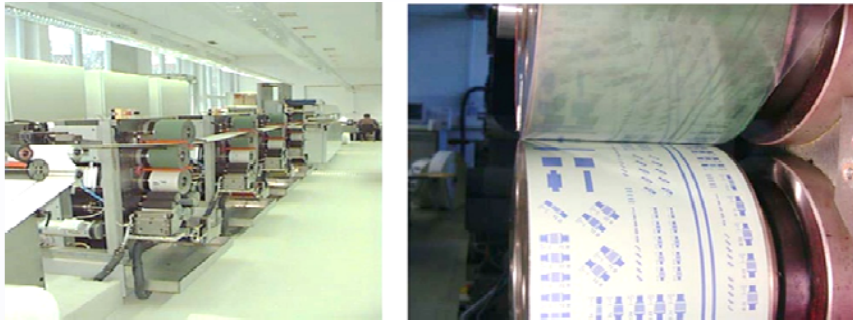
Offset printing machine to produce source/drain structures (D. Zielke et al., Appl. Phys. Lett. 87 (2005) 123508)
