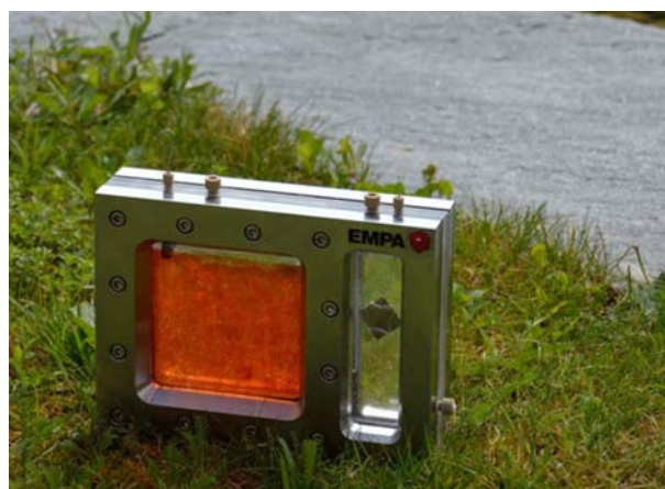
Fig. (6). BioPEC solar hydrogen generator with a hematite-phycocyanin hybrid photoanode (red pane, size: 10 x 10 cm). The hematite layer was deposited on standard fluorine doped tin oxide coated glass. Electrolyte: PBS solution in contact with a platinum counter electrode.
